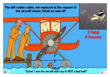
Lack of Assertiveness has been a contributing factor in way too many accidents. Looking at the cartoon takes us back to a fatal float plane accident up North many years ago. A conscious Aircraft Maintenance Engineer (AME) found a corroded rudder cable just inside the empennage on a routine annual inspection. He brought it to the attention
